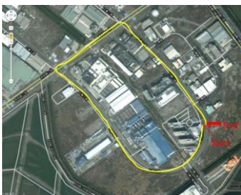
Car speed : 20~60 Km/hr DR horizontal error : 12m (0.6%) (2.0km road distance traveled)
