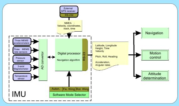
Note: in the standard configuration magnetometer is not used in the navigation algorithm. In order to include it in calculations, a special procedure of deviation compensation must be implemented for each installation type (contact Galaxy for details).
