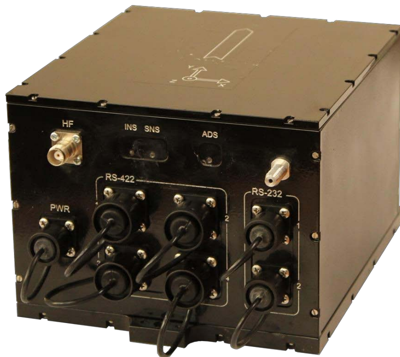
Figure 1. Nav-5L navigation system
